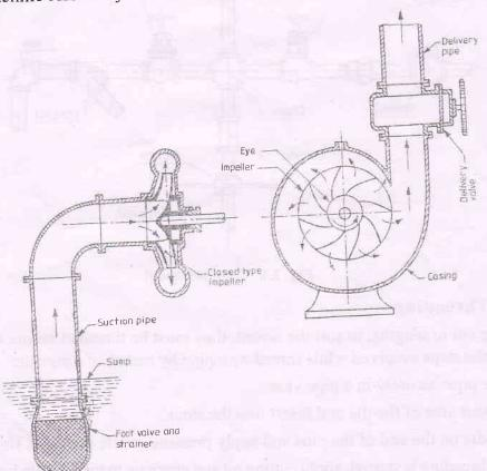
Fig. 2.10 Pipe connections on the suction and delivery sides of a centrifugal pump
