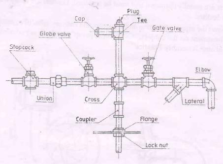
Fig. 2.9 C.I pipe layout
