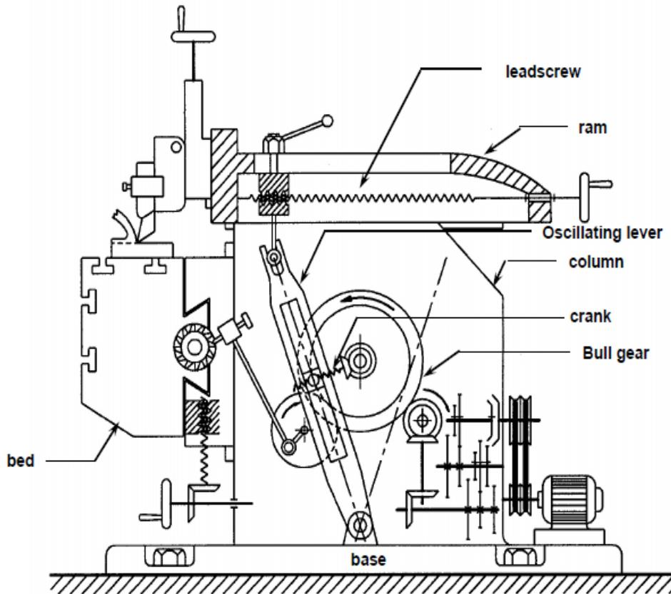
The central large bull gear receives its rotation from the motor through the belt-pulley, clutch, speed gear box and then the pinion. The rotation of the crank causes oscillation of the link and thereby reciprocation of the ram and hence the tool in straight path. Cutting velocity which needs to be varied depending upon the tool-work materials, depends upon
